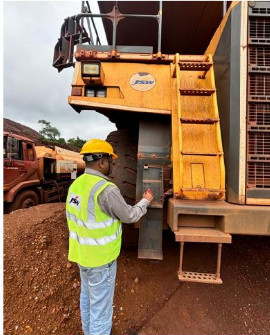
Fig 3: - Battery Cut-off by operator.
