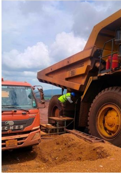
Fig 4: Diesel Refuelling in Dumper.
