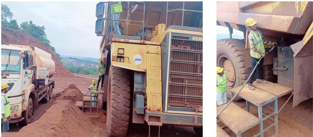
Fig 2: Diesel Filling in Dumper at fixed fueling point.
